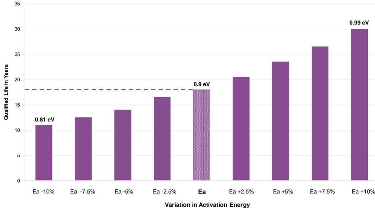
Influence of activation energy on qualified life, determined from artificial thermal ageing for 42 days at 110° C, followed by simulated design basis event. The normal service temperature is 50° C.  $E = 0.9$  eV
