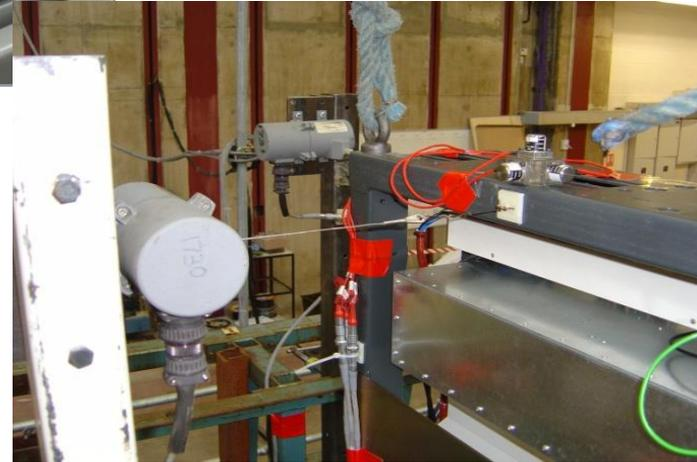
Typically: acceleration, displacement and strain
