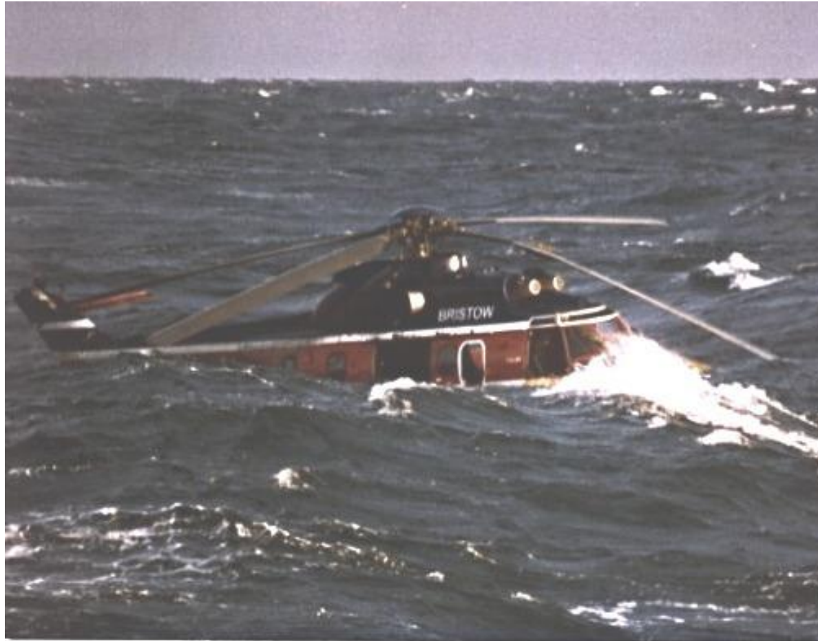
Showing G-TIGK drifting in heavy seas after ditching and evacuation of occupants, with tail rotor/gearbox missing and damaged main rotor blade.
