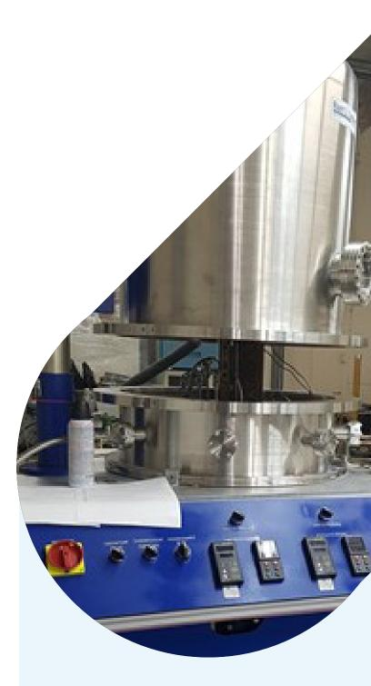
ASTM E595 has become the industry standard test for measuring outgassing properties in organic, polymeric and inorganic materials. In performing the test, material samples such as elastomers, coated parts, seals or composites are placed in a clean standard container. The samples are typically 2mm cubes, but other sizes may be used depending on the material being tested (the minimum size is typically 200 mg).
