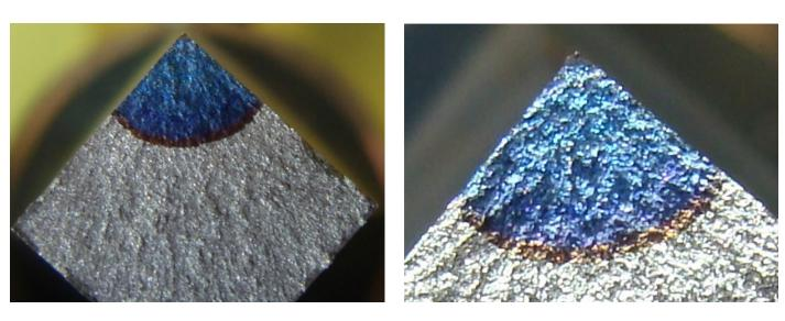
Beachmarks are often observed in fracture faces. They are caused by changes in the load regime or environmental conditions. They are often induced to mark the crack length without damaging the test piece. The images are approximately 10 mm wide.
