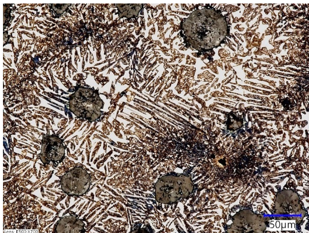
Figure 14. Optical micrograph showing quenched microstructure illustrating the unique lamellar austenite in ferrite structure that had formed by intercritical heat treatment.
